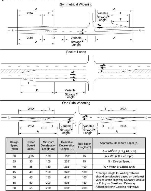
Note: Make every attempt possible to use the desirable deceleration length. It can be shortened as needed but shall not be less than the minimum. Coordinate with NCDOT and get approval on anything less than the desirable deceleration length.
