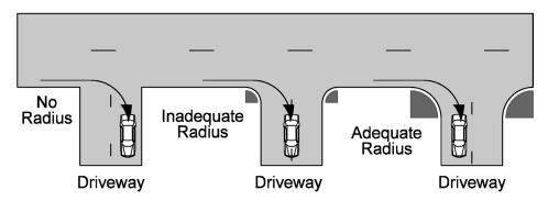
Note: An adequate radius allows turning vehicles to access the site readily and minimizes the impact to the through movement.
