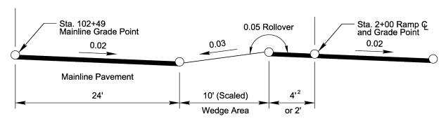
Maximum Elevation Diagram for Ramp Grade at Station 2+00
