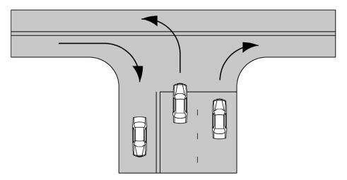
Note: When driveway volumes are moderate or high, a three-lane cross section should be recommended.
