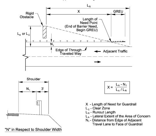
Note: For normal shoulder widths refer to RDM Part I Chapter 4 Section 4.4 Tables 4-1 and 4-2. Note that the width of the shoulder from the edge of travel lane to the face of guardrail increases in certain scenarios as defined in Chapter 4.
