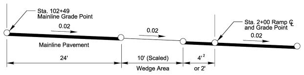
Desirable Elevation Diagram for Ramp Grade at Station 2+00
