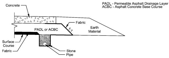
Note: The detail above serves as an example of what a roadway designer may receive from the Pavement Design Unit upon being notified that shoulder drains should be included in the plans.
