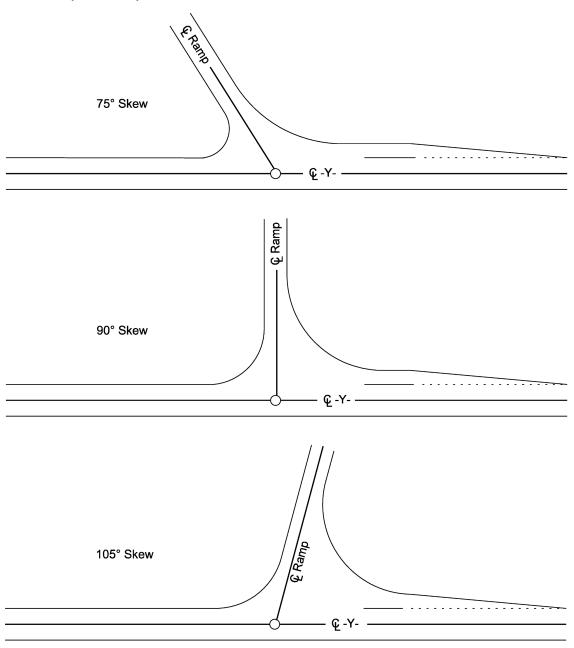
Note:  $90^{\circ}$  is the preferred ramp skew. Anything within the range of  $75^{\circ}$  and  $105^{\circ}$  is considered acceptable.
