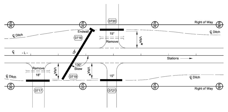
Note: VRA = Vehicle Recovery Area. Refer to RDM Part I Chapter 4 Section 4.6 for the definition of Vehicle Recovery Area.
