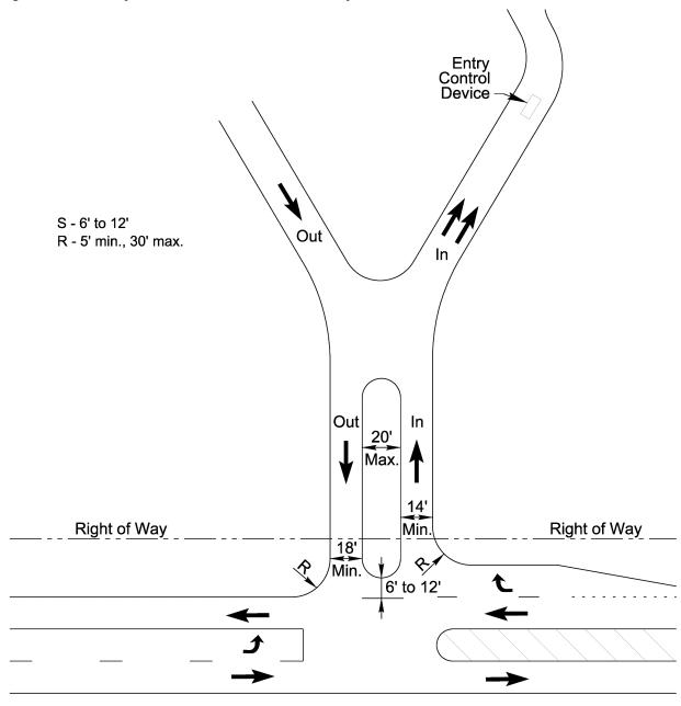
Note: Locate gates, ticket offices or other entry control devices to accommodate peak ingress traffic storage without spill back into the adjacent public street.
