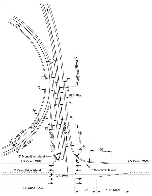
Figure 9-9 Section View for Loop Ramp Terminal Combination
