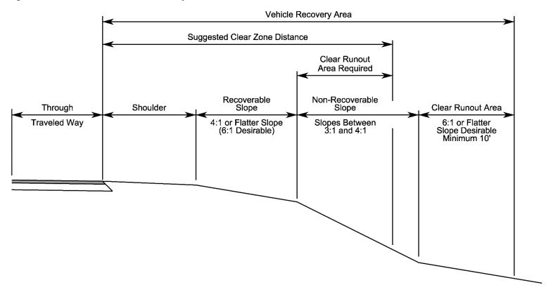
Note: Clear runout area is additional clear zone space that is needed because a portion of the suggested clear zone distance falls on a non-recoverable slope. The width of the clear runout area is equal to that portion of the clear zone distance located on the non-recoverable slope.
