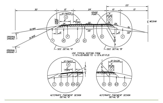
Figure 13-4 Pavement Alternate Base Course Material typical
