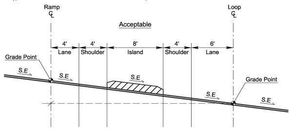
Note: In acceptable scenario the island can be superelevated to match the adjacent roadway cross-slopes.
